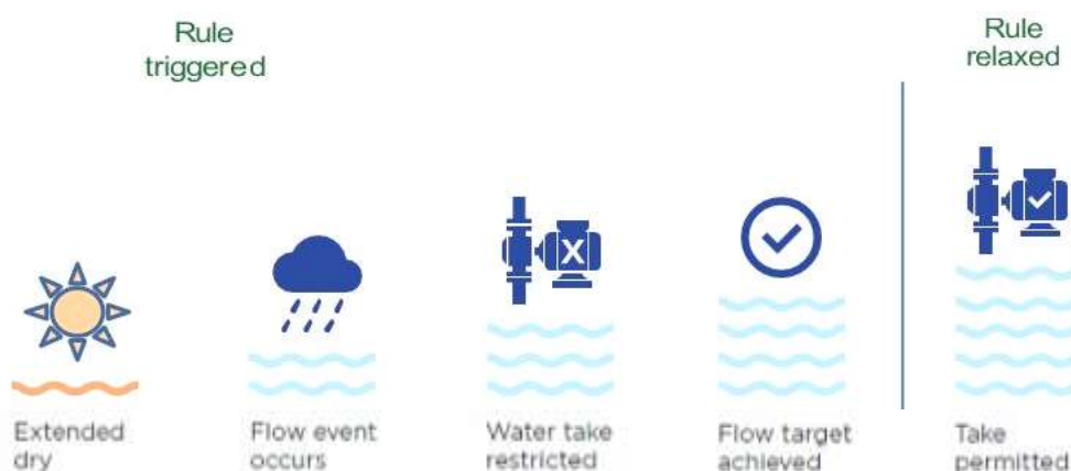
Figure 21: Schematic showing when a resumption of flows rule would be triggered and relaxed 378
